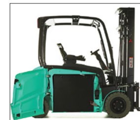
Battery sideways exchange chassis
