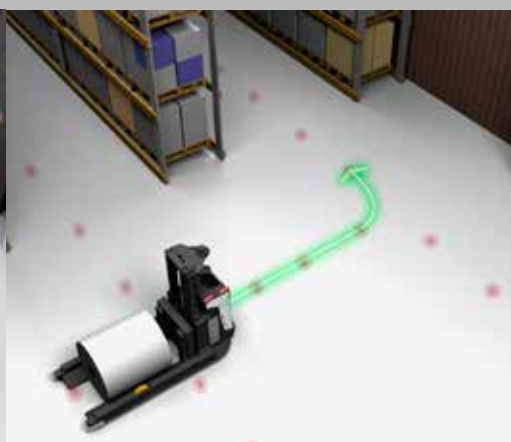
Magnetic spots (for high block storages)
