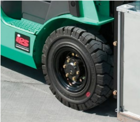
Solid pneumatic dual drive tyres
