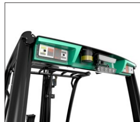
LED working lights, 2 front and 1 rear.
