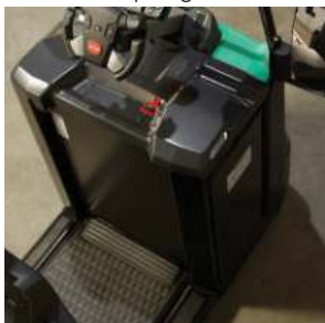
Suspended operator's platform
