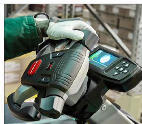
Multifunctional steering wheel with optional color display.
