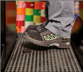
Foot switch for lowering the driver's platform
