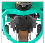
**#7** Double brake discs (1.5 tonne model) enhance braking performance.
